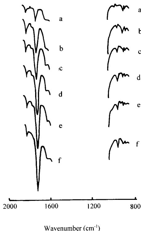
Figure 1 FTIR spectra of electron beam irradiated HDPE at (a) 0, (b) 20, (c) 40, (d) 60, (e) 80, and (f) 100 kGy.
